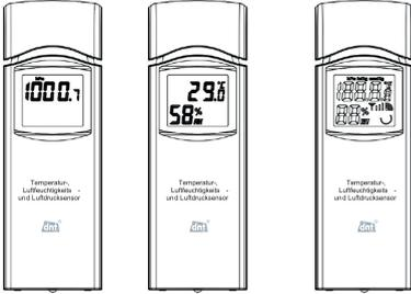
The indoor sensor displays room temperature and humidity, alternatively air pressure for the master sensor.
